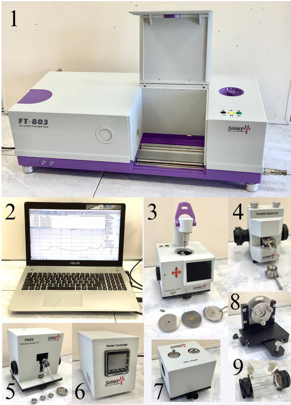
Figure 1. (1) Simex FT-803 infrared Fourier spectrometer with (2) a control computer and a set of set-top boxes: (3) a set-top box with replaceable pads equipped with ZnSe crystals or diamond, (4) cuvettes for liquid samples with an adjustable optical path length, (5) a PRIZE set-top box for analysis solid samples by diffuse reflection/transmission method, (6) temperature control unit for the ATR accessory ; (7) a coupler for connecting fiber-optic probes; (8) set-top box for analyzing films; (9) a gas cell.
