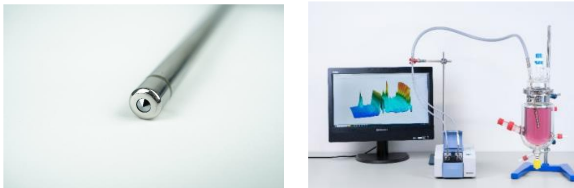
Fig.1 ATR fiber probe. Images courtesy of art photonics GmbH.
